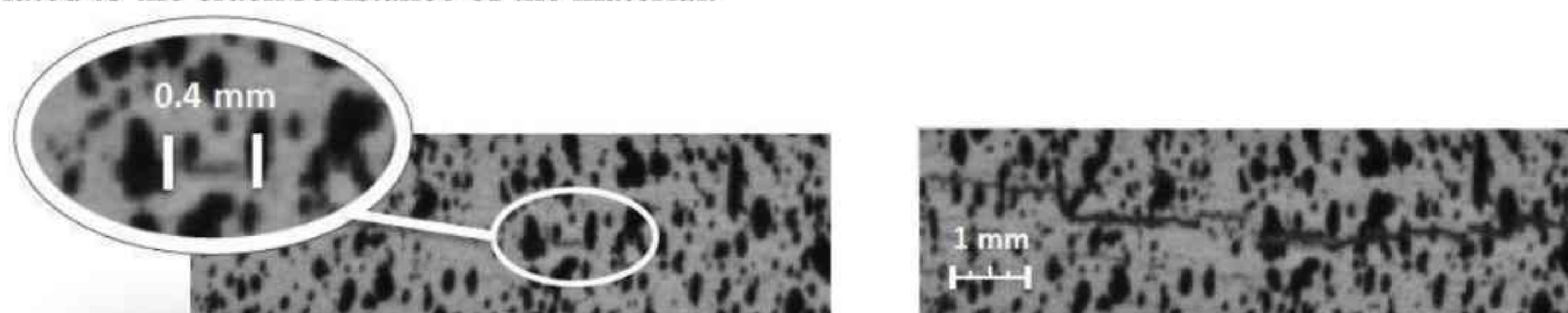
Fig. 5 Left: micro (hairline)-crack vs. Right: macro-crack (same orientation as Fig. 3)
